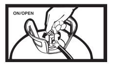
5) Turn the tank valves on fully, noting the initial movement of chemical through the clear hoses as a confirmation of flow.
