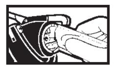
3) Apply a coating of petroleum jelly to the inside face of the *Insta-Flo* dispenser. This makes cleaning of the dispenser face much easier and extends the effective life of the *Insta-Flo* dispenser.
