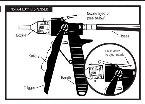
trigger down) and valves CLOSED. Remove used nozzle, reapply petroleum jelly to face of *Insta-Flo* dispenser, and reinsert the used nozzle. Do not bleed pressure off hoses during storage. See Troubleshooting above.
