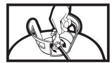
4) For users of Froth-Pak 600 polyurethane foam. Using the wrench provided, tighten the hose assemblies for both "A" and "B" valves until both are tight. The enclosed wrench is intentionally designed to warp or bend if excessive pressure is applied.
