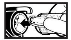
7) Select either a clear (caulking) or blue (spray) Anti-Crossover Nozzle. Insert it firmly into the front of the *Insta-Flo* dispenser. Be sure the dispenser clips the nozzle firmly in place.
