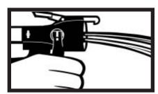
6) Purge the system into a waste container by activating the trigger of the *Insta-Flo* dispenser. When streams are equal, release the trigger, clean the chemical from the dispenser face with a clean rag, and reapply petroleum jelly.
