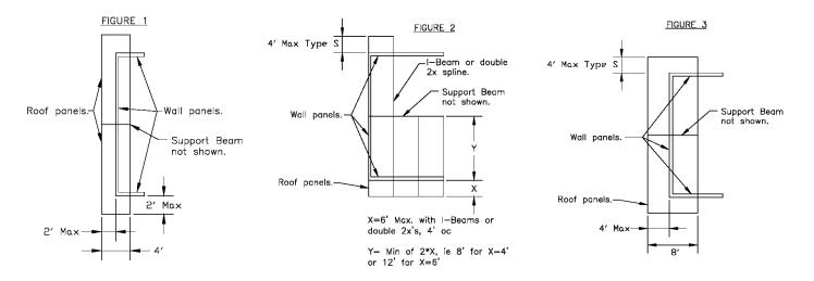
Extreme Panels used to create overhangs on gable end walls or on eave applications where the panel is parallel to the support wall can be used up to 2' in unsupported overhangs (FIGURE 1). Panels used parallel to the support wall can support loads indicated in the "Cantilevered Roof Panels Parallel to Support Wall – Type "S" Panel Capacity" load chart shown below.
