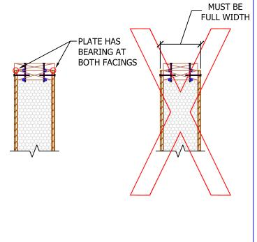
DO NOT HAVE UNSUPPORTED HORIZONTAL JOINTS IN WALL UNLESS SPECIFIC CONDITION IS DESIGNED BY A LICENSED STRUCTURAL ENGINEER. I.E. DON'T STACK WALLS.
