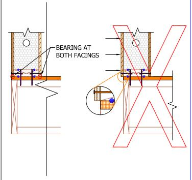
BOTH SIP WALL FACINGS CANNOT COME IN DIRECT CONTACT WITH CONCRETE. BEST PRACTICE IS TO USE A TREATED SILL PLATE BETWEEN CONCRETE AND BOTH SIP FACINGS. THERE MUST BE A CAPILLARY BREAK BETWEEN CONCRETE AND BOTH SIP FACINGS.
