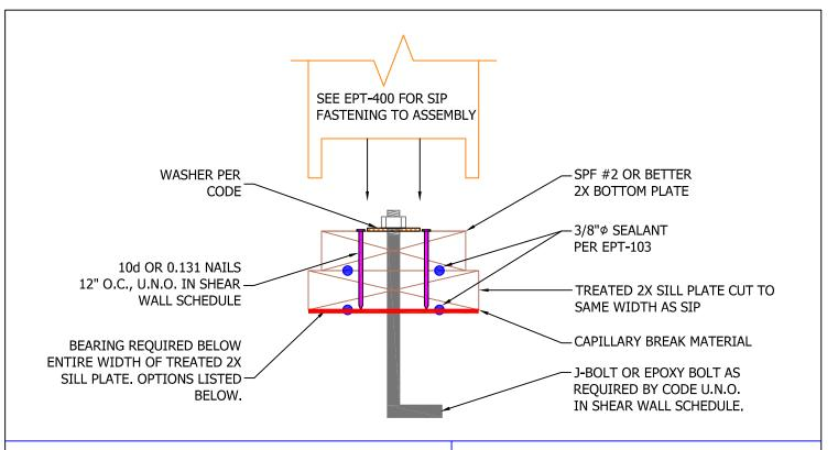
A: CANTILEVERED STRUCTURAL SILL PLATE
