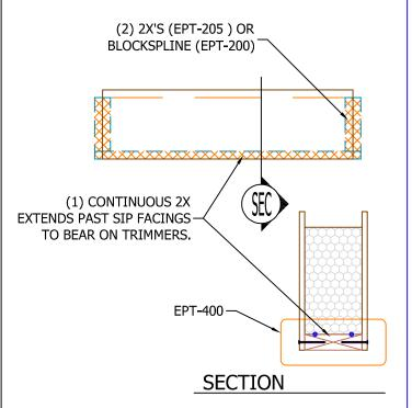
IHDR-1 PLY: INSULATED HEADER (1) PLY LVL. SEE EPT-407 OR EPT-408 FOR ASSEMBLY SEQUENCE.
