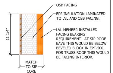
IHDR-2 PLY: INSULATED HEADER (2) PLY LVL. SEE EPT-407 OR EPT-408 FOR ASSEMBLY SEQUENCE.
