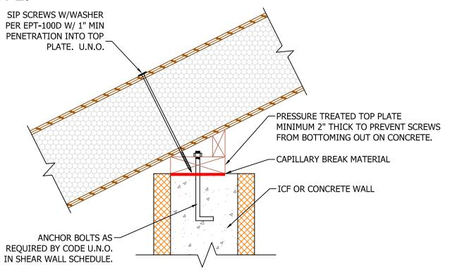
STRUCTURAL SUPPORT TO PROVIDE 1 1/2" MIN. BEARING FOR SIP
