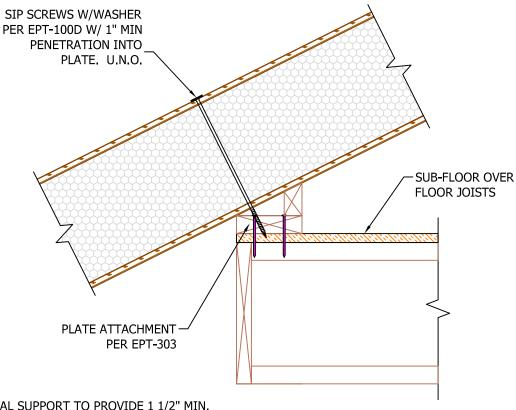
STRUCTURAL SUPPORT TO PROVIDE 1 1/2" MIN. BEARING FOR SIP
